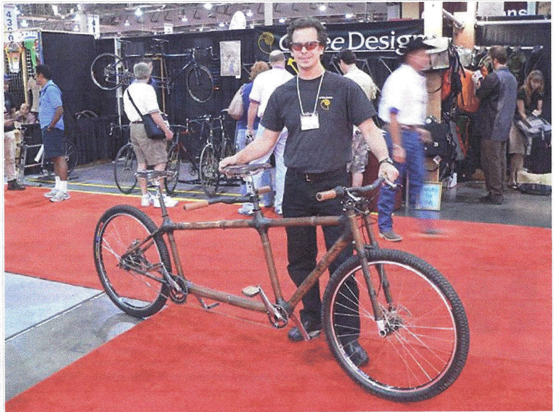
Craig Calfee poses with his bamboo and carbon fiber wunder-tandem. Photo ©: James Huang/Cyclingnews
