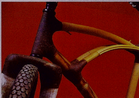
In his bicycle frames, Craig Calfee uses bamboo stalks that are naturally formed to balance stiffness and vibration dampening
